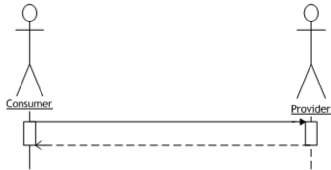
Figure 3-4 Synchronous Request/Response Sequence
