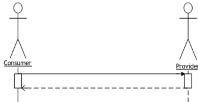
Figure 3-4 Synchronous Request/Response Sequence
